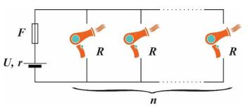
electric fuse F with a negligible resistance. Electric fuse is a special element used in electric circuits in order to limit the máximum electric current allowed. When the current reaches the máximum value fuse blows, behaving like an open switch thus disabling the current flow. Maximum electric current allowed by the fuse Ivan and Aleksandra used in their hair salón is  $I_{\rm kr} = 16 \,\text{A}$ .
